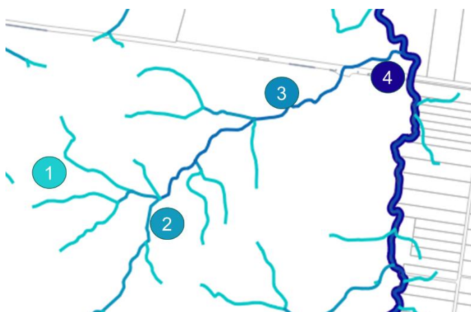
How Strahler order creeks are categorised, with the lightest coloured lines representing the smallest creeks.
